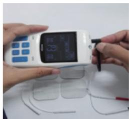
into the receptacle on the top of the main device. Ensure the electrode wires are inserted correctly. The device has two output receptacles controlled by Channel A and Channel B at the top of the unit. You may choose to use one channel with one pair of electrode wires or both channels with two pairs of electrode wires. Using both channels gives the user the advantage of stimulating two different areas at the same time.
