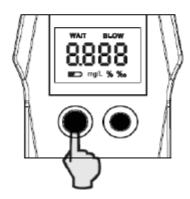
LCD will display test counter before starting countdown.
